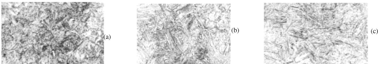
Fig. 3. The appearance of structure after quenching with austenitising of material at 930^\circ\text{C} (a) steel 1 micro-alloyed with Nb; (b) steel 2 microalloyed with both Nb and V (c) steel 3 microalloyed with Mo
